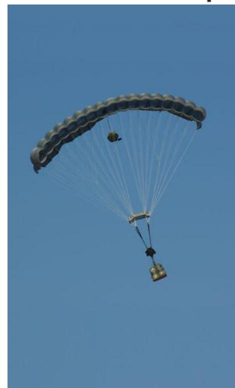
**Sherpa™** can be easily integrated with different types of cargo payloads, including standardized Container Delivery Systems (CDS) designed for aerial delivery on military aircraft. Sherpa has been successfully deployed with various platforms such as 463L, Type-V, Enhanced Container Delivery Systems (ECDS), Low Cost Containers (LCC) and custom payloads, including Special Operations Combat Expendable Payloads (SOCXP).
